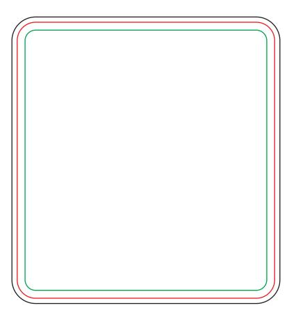
Red line is the die cut Green line is the 3mm safety net Black line is 2mm bleed
